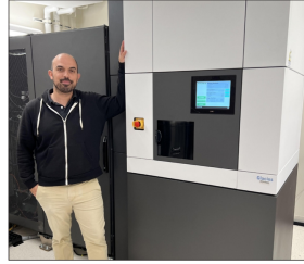
UCSC's research specialist, Vitor Hugo Balasco Serrão, stands with the Glacios cryo-electron microscope. The microscope uses electrons, instead of light, to capture pictures of frozen proteins. ELISE OVERGAARD — SANTA CRUZ SENTINEL
